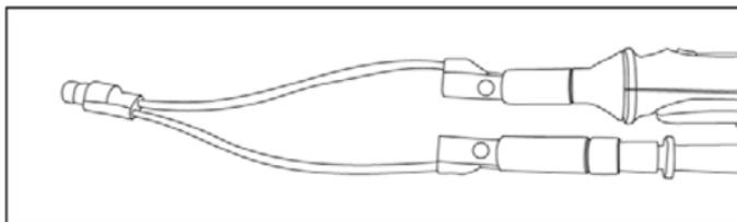
**NOTE:** The BNC adaptor does not make the Pokit Pro compatible with oscilloscope leads. Oscilloscope leads contain a series resistance which will interfere with the voltage measurement circuitry inside the Pokit Pro.
